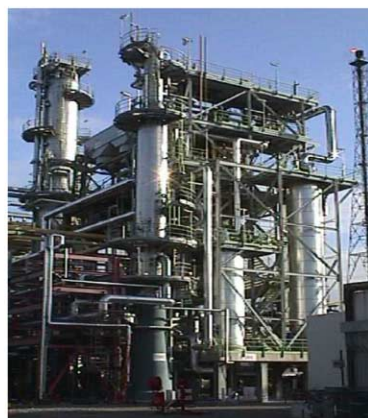
Fig. 5. SCANfining II enables deep HDS of high sulfur feeds with reduced octane loss.
